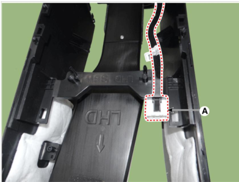
5. Remove the console rear cover (A) after loosening the mounting screws.
