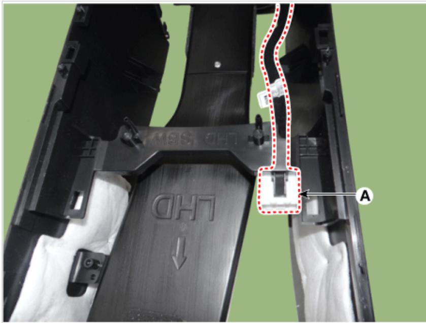
5. Remove the console rear cover (A) after loosening the mounting screws.
